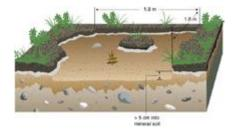
Wide gouges are excavations into mineral soil that are a) deeper than 5 cm at the survey point and b) deeper than 5 cm or to bedrock, on at least 80% of an area 1.8 x 1.8 m.
