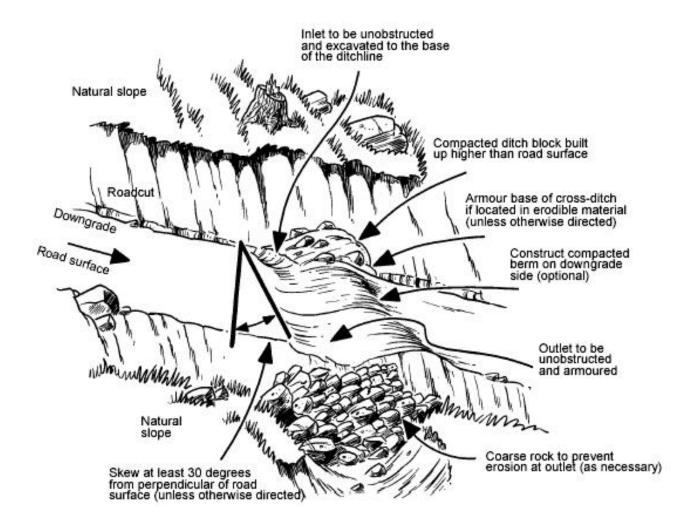
A well-compacted ditch block will be installed immediately downgrade of the cross-ditch inlet. The ditch block is usually higher than the road surface. The ditch block should be non-erodible, relatively impermeable, and large enough to divert all expected flows into the cross-ditch. Where ditchwater converges at low points in the road, no ditch block or berm is required, as the cross-ditch should be constructed as a broad gentle swale.
